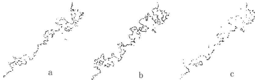
Figure 6. The distribution of GCPs obtained by CR match technique from two sequential SeaWiFS images (a), that from two AVHRR images (b), and that from SeaWiFS image and AVHRR image (c). Only the points in the second image are shown.
